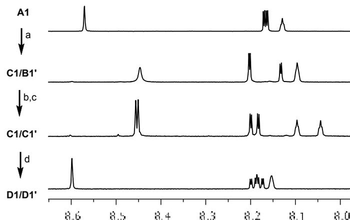
NMR expansion of downfield aromatic and imine protons for steps a-d. From left to right, imine protons, *meta* ester protons, *meta* imine (carbon side) singlet.
