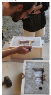
Fig. 2: Participants of the workshop preparing sand moulds for the aluminum casting exercice.
