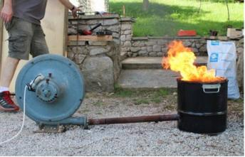
Fig. 17: Aluminum melting oven
