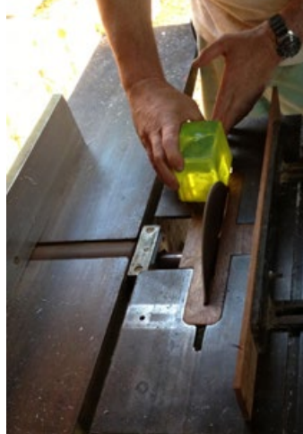
Fig. 26: Carpentry table saw.
