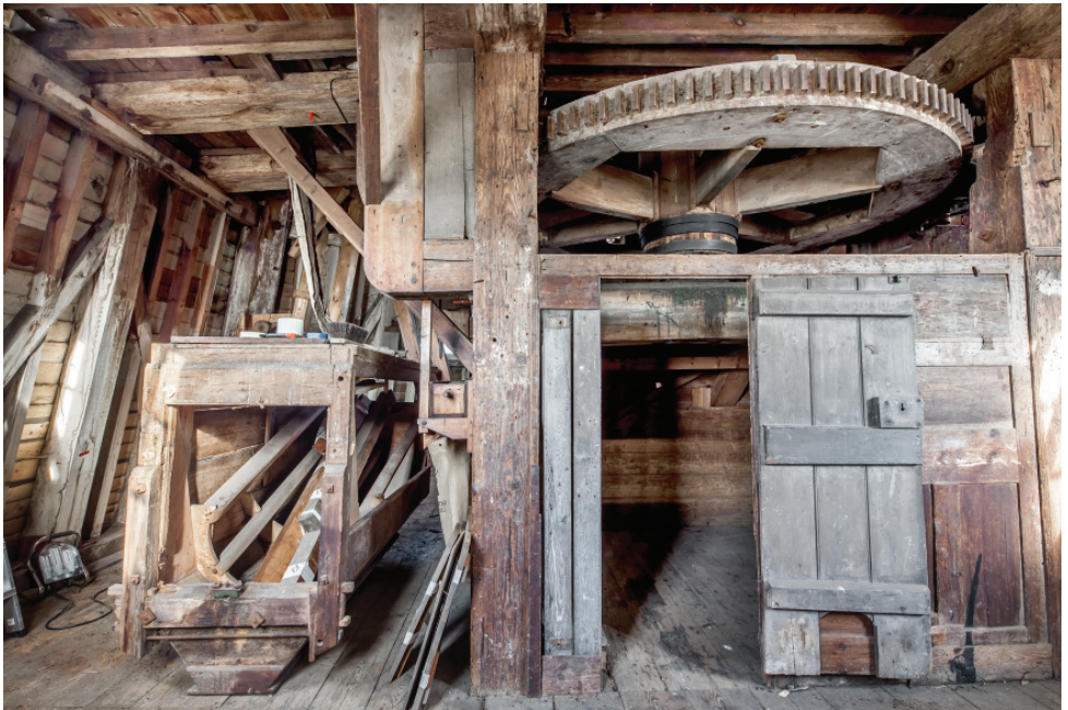
Bolter on the Meal Floor moved away from the wall
