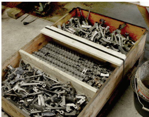
7. Shutter hinges, plain and with levers.
