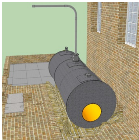
Left: The boiler shell sat above flues built into the floor. Right: The fire tube and sides of the shell were enclosed to direct hot exhaust gasses into the under flues to give added heating.
