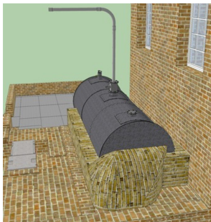
Left: The boiler shell sat above flues built into the floor. Right: The fire tube and sides of the shell were enclosed to direct hot exhaust gasses into the under flues to give added heating.
