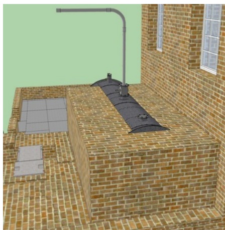
Left: Outer brick enclosure. Right: The face of the boiler protruded into the Coal House for stoking. Two iron trapdoors provided access to the under flues for cleaning.
