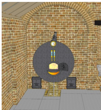
Left: Outer brick enclosure. Right: The face of the boiler protruded into the Coal House for stoking. Two iron trapdoors provided access to the under flues for cleaning.
