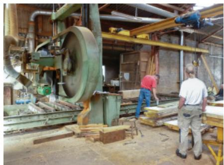
Giant saw that will be used to cut the pine logs down for the corner posts
