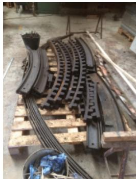
Sections of the iron curb channels and gear rack
