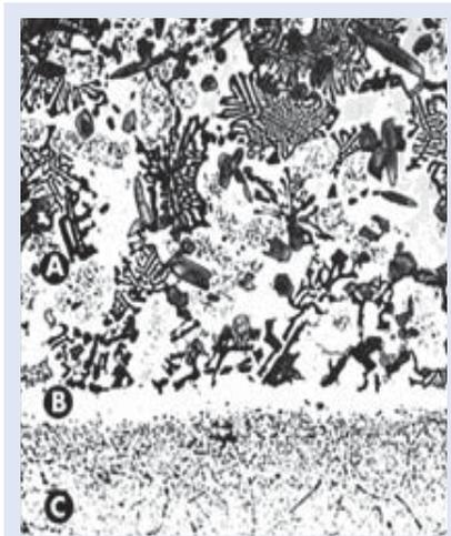
Metallurgical bonding with no dilution of Eutalloy® alloy, on stainless steel (enlarged x 500).
