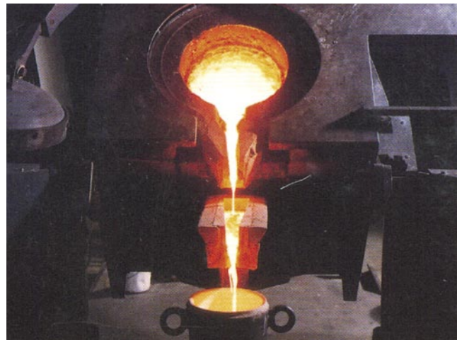
Molten alloy being poured into the gas-atomization chamber. Making our own powders ensures the quality needed for the best coating performance.
