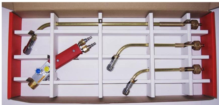
The CastoFuse® kit consists of a handgrip with three fusion lances 20, 30 and 40. The kit's three lances offer different flame powers, so work pieces of different mass or thickness can be preheated and heated up to the coating fusion temperature.
