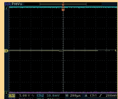
353 ECV Arc Power Supply Fluctuation ( \pm 200 mV)
