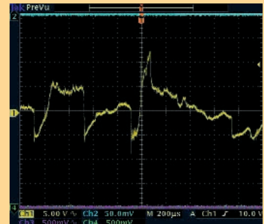
Standard Arc Power Supply Fluctuation ( \pm 10 V)
