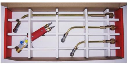
The CastoFuse® kit consists of a handgrip with three fusion lances 20, 30 and 40. The kit's three lances offer different flame powers, so work pieces of different mas or thickness can be preheated and heated up to the coating fusion temperature.
